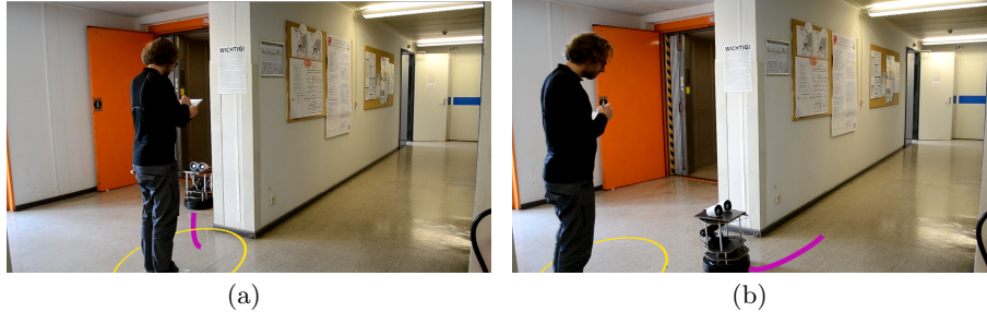
Fig. 1. (a) As soon as the local path plan (pink) overlaps the personal space (yellow) the robot starts to say “Excuse me, I need to pass urgently to rescue a patient in the other corridor – thank you.” (b) However, as the person steps aside the robot leaves personal space before the whole explanation was uttered resulting in “Excuse me, I need to pass urgently – thank you.”
