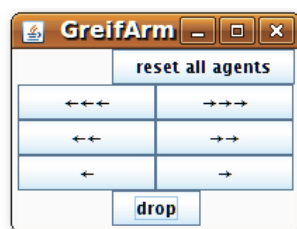
Figure 5.16: Graphical wizard interface for the robot arm domain; stopping was realized as moving a tiny distance into the opposite direction.
